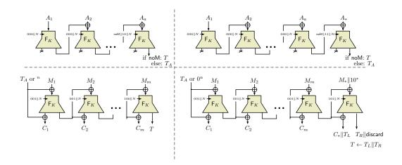
**Figure 12:** The encryption algorithm of SAEF[F] mode. The bit noM = 1 iff |M| = 0. The picture illustrates the processing of AD when length of AD is a multiple of n (top left) and when the length of AD is not a multiple of n (top right), and the processing of the message when length of the message is a multiple of n (bottom left) and when the length of message is not a multiple of n (bottom right)
