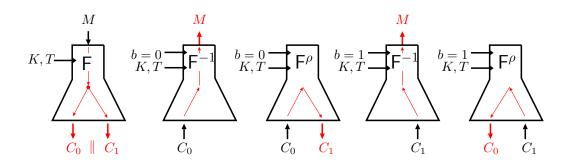
Figure 4: Forward and backward execution of a forkcipher.
