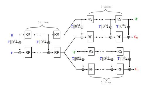
**Figure 2:** Illustration of an encryption by ForkAES. A 128 bit plaintext P, a 128 bit key K and 64 bit tweak T (all in blue) are used to compute a 256 bit ciphertext  $C = C_0 ||C_1|$  (in red). RF denotes a single iteration of the AES round function and KS denotes a single iteration of the AES keyschedule.
