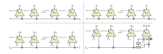
**Figure 9:** The encryption algorithm of PAEF[F] mode. The picture illustrates the processing of AD when length of AD is a multiple of n (**top left**) and when the length of AD is not a multiple of n (**top right**), and the processing of the message when length of the message is a multiple of n (**bottom left**) and when the length of message is not a multiple of n (**bottom right**)
