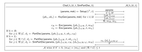
Fig. 2: Static Partial Decryption Simulatability Game for Threshold Encryption
