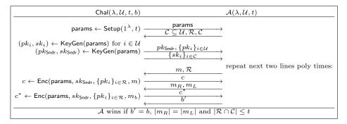
Fig. 13: Super-Static Semantic Security Game for Keyed-Sender Ad Hoc Threshold Encryption.
