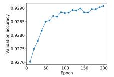
**Fig. 1.** Training a neural network to distinguish 5-round Speck32/64 output for the input difference  $\Delta = 0x0040/0$  from random data. (*left*) Training and validation loss by epoch. (*right*) Validation accuracy. (*both*) Only data for epochs with lowest learning rate is shown. Intermediate epochs contained excursions to low performance. Full learning history for this run is available from supplementary data.
