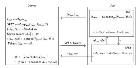
Fig. 6. Diagram of our payment scheme. The hardware calculates the value  $\sigma$  via the Eval<sub>HW</sub> function on input  $id_{tk}$ , the label and the master key. WPAY executes the Check<sub>SW</sub> function on input  $\sigma$  and on the sub-key and  $id_{tk}$ .
