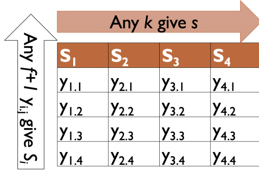
Fig. 1. Intuition of HAVSS. P_j receives row y_{*,j} which is used to compute the recovery polynomial b_j(y) and column y_{j,*} which is used to compute the share polynomial a_j(x) and recover its share S_j = a_j(0) . If a malicious dealer does not send P_m its share, P_m can still complete indirectly the sharing. This is possible because P_j , that completes the sharing directly, will send P_m a message with y_{m,j} . Since there are f + 1 available parties that should have shares in column m and complete the sharing directly, P_m will get enough points to recover a_j(x) , hence recover S_m = a_m(0) . As a result, eventually k parties will have shares S_i , compute locally u(0, x) and recover the secret s = u(0, 0) .
