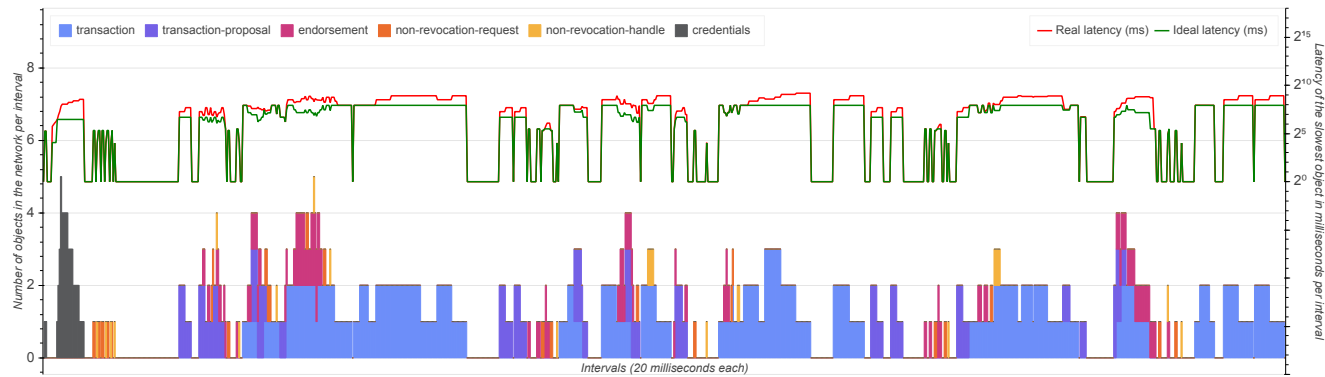
Figure 2: Network log visualization (subset is shown, 18 transactions). Interval size is 20 ms. Simulation involves 5 users, 3 peers, 2 endorsements, 20 KiB/s and 50 KiB/s local and global bandwidths, and epoch length 5 seconds. Bars show objects in the network, lines show latencies. Latency scale is logarithmic.
