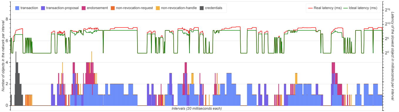
Fig. 3: Network log visualization (subset is shown, 18 transactions). Interval size is 20 ms. Experiment involves 5 users, 3 peers, 2 endorsements, 20 KiB/s and 50 KiB/s local and global bandwidths, and epoch length 5 seconds. Bars show objects in the network, lines show latencies (green for ideal, red for real). Latency scale is logarithmic.
