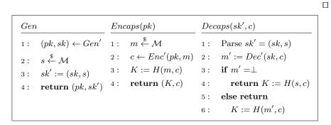
Fig. 22: IND-CCA-secure KEM-III =  $U^{\not\perp}[PKE', H]$
