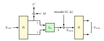
Figure 1: Illustration of the feedback process for a message block M of |M| bits. Here  $encode(M, \Delta)$  represents some encoding of |M| bits string to a b-bit string as described above and  $L_e$  is a linear transformation applied on b-bit strings.
