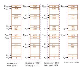
Fig. 3. Memory access during two-core NTT.
