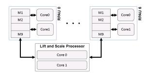
Fig. 10. Block diagram of coprocessor for computing homomorphic operations
