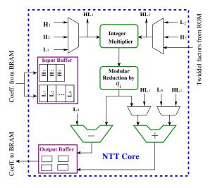
Fig. 4. Architecture of NTT Core.
