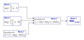
Fig. 9. Architecture of Scale  $Q \rightarrow q$  using small number arithmetic.
