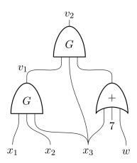
**Circuit.** An example circuit  $C(x_1, x_2, x_3, w)$  using an arbitrary three-input G-gate. The circuit takes as input the vector  $(x_1, x_2, x_3) \in \mathbb{F}^3$ , and a witness  $w \in \mathbb{F}$ . The circuit C outputs  $v_2$ , the value on the output wire of the topologically last G-gate.
