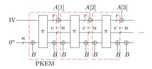
Fig. 5: The PKEM-based representation of a keyed sponge with  $\kappa$ -bit key/initial seed B. Inside the red dashed rectangles are the "partial-key" Even-Mansour cipher. It's easy to see after the internal actions of XORing B cancel, the construction turns basically the same as the keyed sponge.
