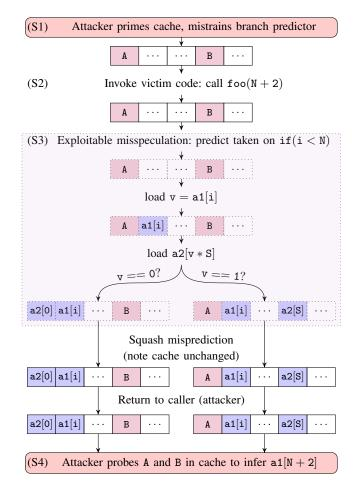
Figure 2: Cache state evolution in Spectre variant 1. The rectangular boxes show the addresses that are cached. Untrusted accesses are red while accesses by trusted code are blue. For simplicity, we show the attack on a direct-mapped cache. The extension to set associative caches is straightforward.
