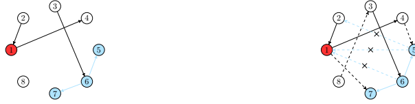
Figure 1: An example directed re-encryption graph, \mathcal{DRG} . If a challenge is learned under \text{pk}_6 and \mathcal{A} has learned tokens \Delta_{6,5} and \Delta_{6,7} , then \text{pk}_5, \text{pk}_6 are also considered challenge keys . Therefore, token queries that lead to paths from challenge keys to corrupted ones such as \Delta_{6,1} or \Delta_{5,2} result in a trivial win. The graph on the right gives some examples of what tokens the adversary can and cannot learn next.
