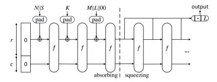
Figure 4: Construction of KMAC
