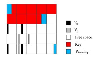
Figure 9: The Initial State of KETJE SR v1
