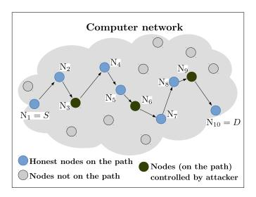
Fig. 1: A network path between the source node S and the destination node D.
