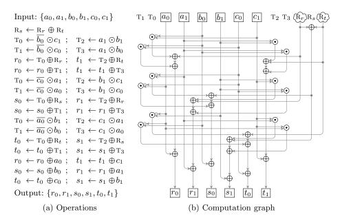
Fig. 10: Single-fault SIFA-resistant  $\chi_3$  using 2 shares, with global checks.
