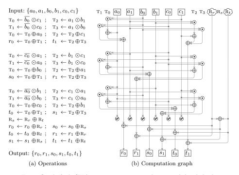
Fig. 9: Single-fault SIFA-resistant  $\chi_3$  using 2 shares, with local checks.
