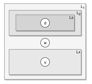
**Figure 10.** Conversion Point (min-cut): The conversion point (min-cut) for d (in  $L_3$ ) and u (in  $L_4$ ) is in their closest enclosing block  $L_1$ . w is one node where we can place conversion.
