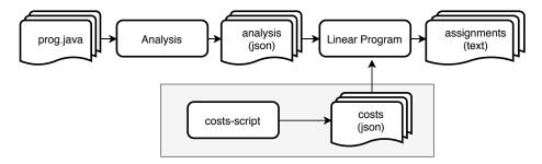
**Figure 4.** Implementation Overview: The analysis takes a Java program as input and outputs a def-use graph (along with related information). The linear program takes as input analysis information and costs, and outputs the optimal assignment.
