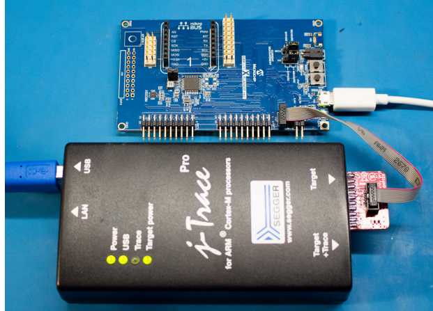
Figure 15: Power analysis using a the on-board ADC with the Microchip SAM L11 Xplained Pro.
