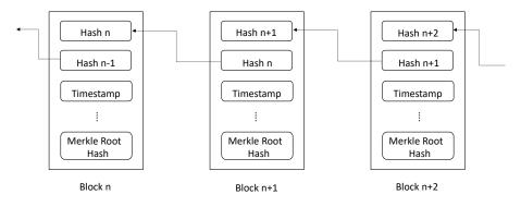
Figure 1: Basic blockchain structure.
