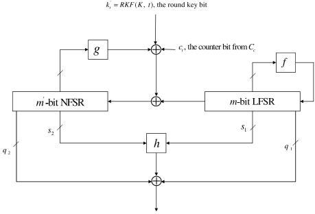
Fig. 1. The generic model for the Grain-like small state stream ciphers
