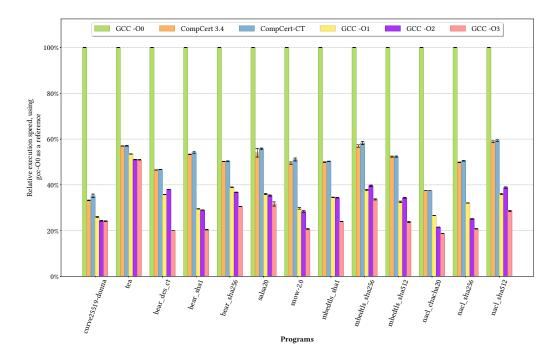
Fig. 10. Relative execution times of our benchmark. We compare the original CompCert, our modified CompCert, and gcc from -00 to -03. We normalized the measured execution times with the execution times of gcc -00. The error bars represent the 99% confidence intervals of our measurements.
