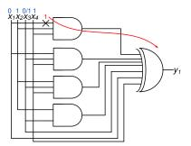
Fig. 3: Fault propagation through S-Box Polynomials. The input pattern causing the propagation is shown in blue. The stuck-at fault type is shown in red numbers.
