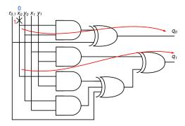
Fig. 4: Fault propagation through masked AND gate.
