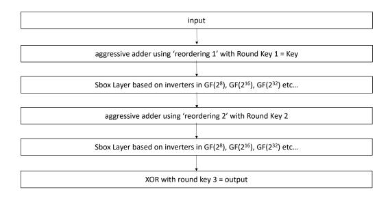
Figure 2: Two Round K-Cipher Specification
