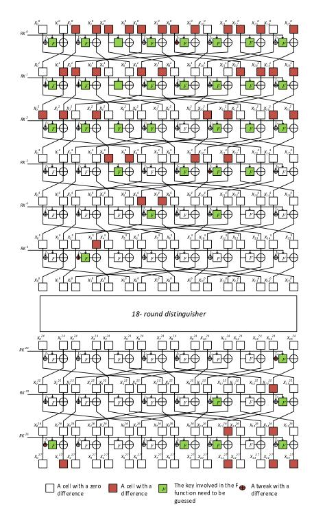
Fig. 3. Impossible differential attack on 27-round T-TWINE-128
