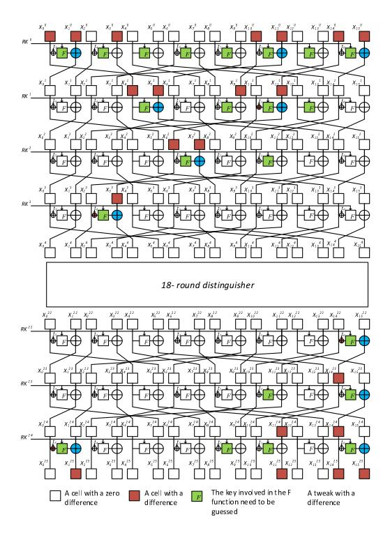
Fig. 4. Impossible differential attack on 25-round T-TWINE-80
