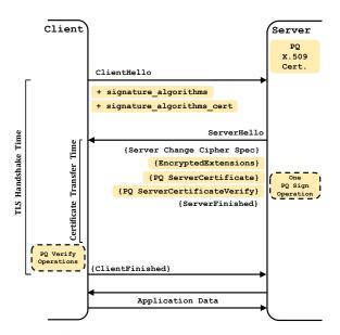
Fig. 2: Post-Quantum TLS 1.3 Handshake
