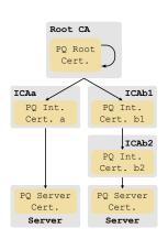
Fig. 5: X.509 certificate chains in our experiments
