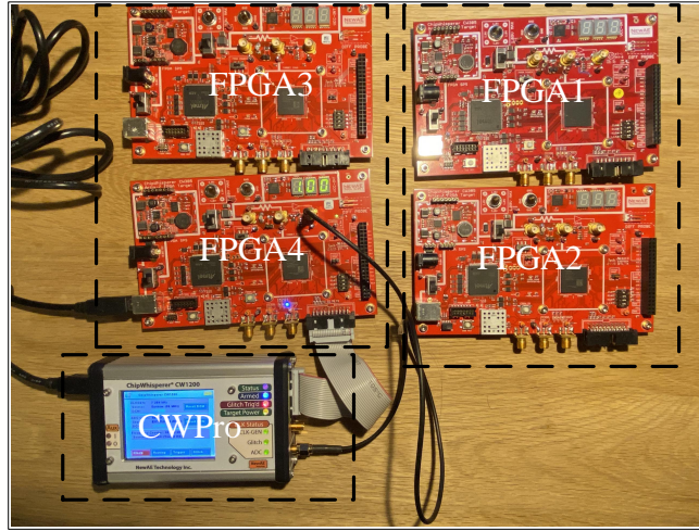
Fig. 2. Equipment for power analysis.
