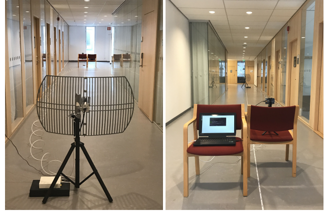
Figure 2: Experimental setup for 15 m distance to target. Photo credit: Katerina Gurova.
