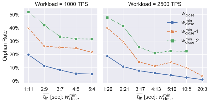
Fig. 8: The orphan rate increases when w_{\text{close}} < w_{\text{close}}^{\min} .
