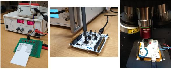
(a) Voltage glitch on a smart (b) Electromagnetic pulse injection on a mi- (c) LASER fault injection on a card crocontroller microcontroller
