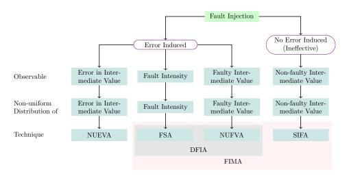
Fig. 8: Overview of statistics based fault analysis methods
