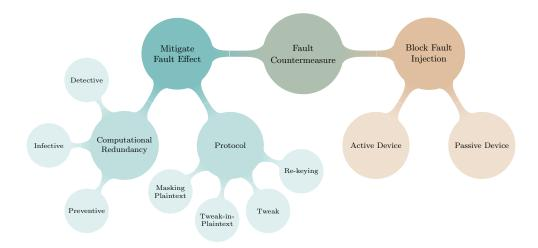
Fig. 9: Generic overview of fault attack countermeasures
