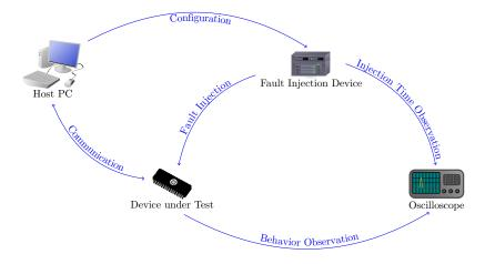
Fig. 2: Schematic view of a fault injection set-up
