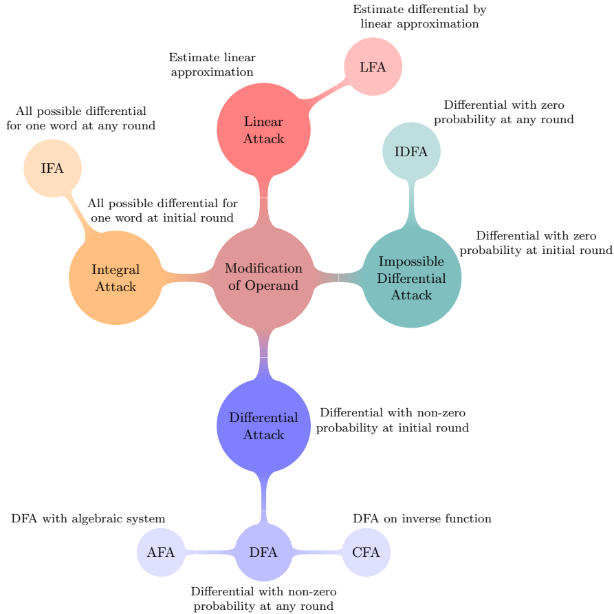
Fig. 1: Attacks (classical and fault) based on modification of operand models
