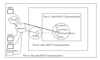
Fig. 1. Three Tier Communication Architecture
