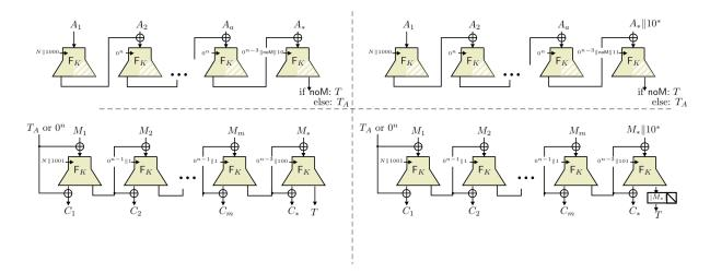
Fig. 1: The encryption algorithm of SAEF[F] mode. The bit noM = 1 iff |M| = 0. The picture illustrates the processing of AD when length of AD is a multiple of n (top left) and when the length of AD is not a multiple of n (top right), and the processing of the message when length of the message is a multiple of n (bottom left) and when the length of message is not a multiple of n (bottom right). The white hatching denotes that an output block is not computed.
