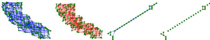
Fig. 6: (Left) Reconstructed dominance graph (blue edges) and anti-dominance graph (red edges) of 200 randomly chosen points from the California Road Network dataset. (Right) The dominance and anti-dominance graphs for the order reconstruction of 08/31/2009 from the Malte Spitz dataset.
