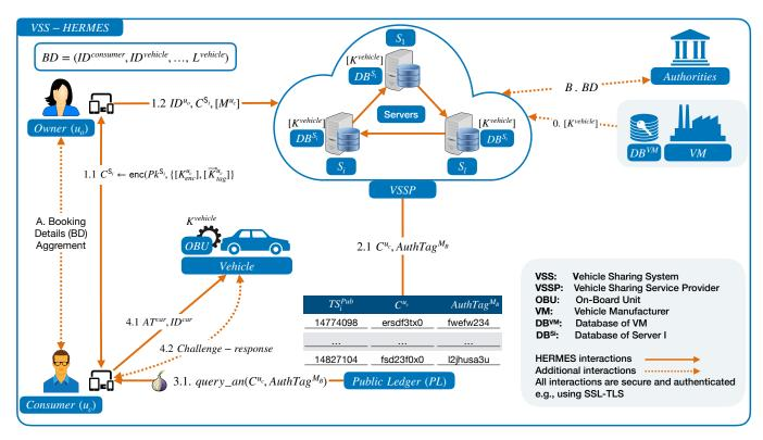
Fig. 2: HERMES high level overview. Numbers correspond to the steps outlined in the text of Section IV. Figures 3, 4, 5 and 6 describe steps 1, 2, 3 and 4 in more detail.
