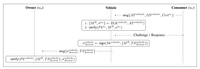
Fig. 6: Step 4: vehicle access. Dashed lines represent close range wireless communication.
