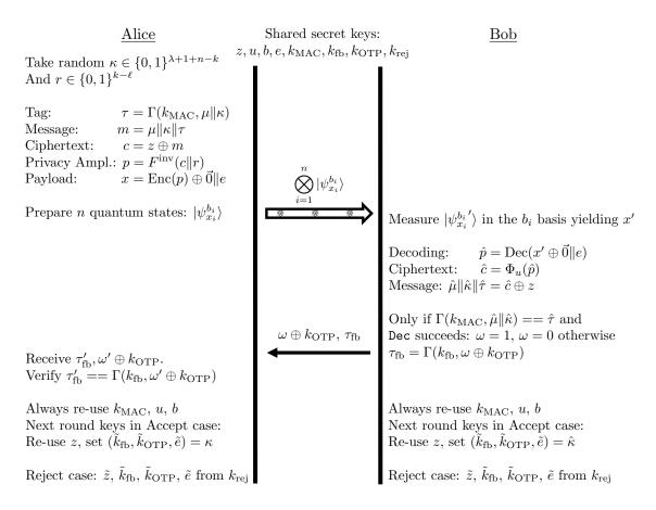
Figure 1: Protocol steps of the 'Embedded' variant.
