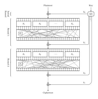
Fig. 1: Quasigroup substitution permutation network
