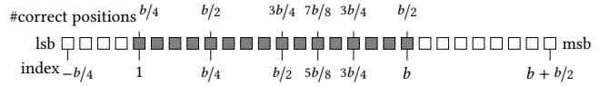
Figure 5: Distribution of correct positions for j \in [1 : b] with e = b/2 and e_p = b/4 .
