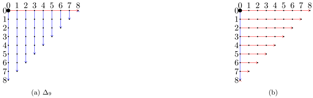
Figure 3: Two basic strategies for computing a degree- \ell^9 isogeny. Subfigures 3a-3b illustrate a multiplicative-oriented approach and an isogeny-oriented approach, respectively. Vertical blue lines indicate scalar multiplications by \ell , whereas horizontal red lines indicate degree- \ell isogeny evaluations.
