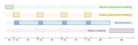
**Figure 4:** Timeline of polynomial multiplication when the public polynomial has 13 bit coefficients, from input loading to output reading. Darker blue areas denote when the multiplier reads coefficients from the loading data instead of the end of the buffer.
