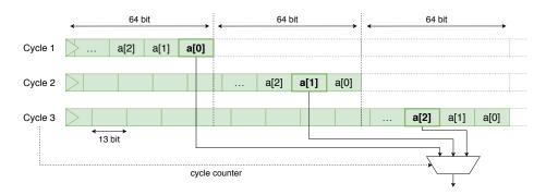
**Figure 3:** Buffer loading of polynomial data for the first three cycles. Each row represents the buffer at different cycles, and green indicates the polynomial data that has been loaded.
