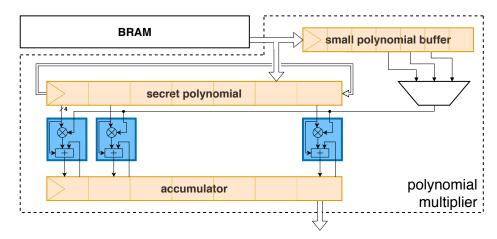
**Figure 2:** The polynomial multiplier architecture. Blue blocks denote processing units, orange blocks are registers and wide arrows represent 64-bit input/output to the multiplier.
