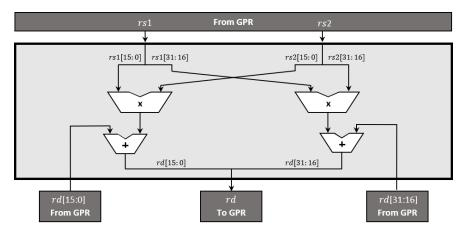
Figure 4: Vectorized Modulo Multiply Accumulate (pq.mac)
