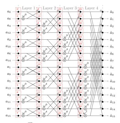
**Figure 9:** Example  $NTT_{br \leftarrow no}^{CT}$  with n = 16 (unoptimized). In this case, one coefficient is stored in a single memory word, two coefficients can be loaded to the register file (l = 2), and one pair of coefficients can be executed in parallel. The red boxes indicate which coefficients are stored together in one word (in this case they are not stored together) and in which order the coefficients are processed by a single butterfly unit.
