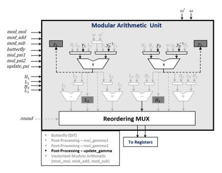
**Figure 10:** Modular Arithmetic Unit – Post-Processing Operation (*mul\_gamma1*, *mul\_gamma2*, *update\_gamma*)
