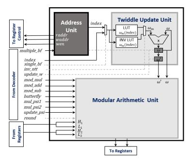
Figure 2: NTT and Modular Arithmetic Unit
