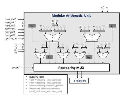
Figure 3: Modular Arithmetic Unit – Butterfly Operation decimation-in-time (DIT)
