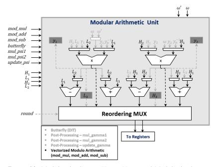
Figure 11: Modular Arithmetic Unit – Vectorized Modulo Arithmetic
