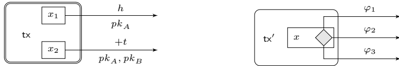
Fig. 1. (Left) \text{tx} is published on the blockchain. The output of value x_1 can be spent by a transaction containing a preimage of h and signed w.r.t. pk_A . The output of value x_2 can be spent by a transaction signed w.r.t. pk_A and pk_B but only if at least t rounds passed since \text{tx} was accepted by the blockchain. (Right) \text{tx}' is not published yet. Its only output can be spent by a transaction whose witness satisfies \varphi_1 \vee \varphi_2 \vee \varphi_3 .
