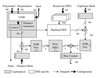
Figure 8: Architecture of a cryptanalytic core.
