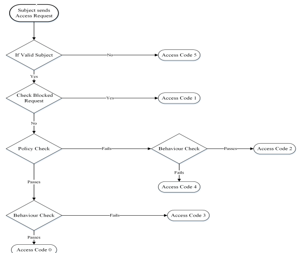
Fig. 3: Execution Flow of Rep-ACM
