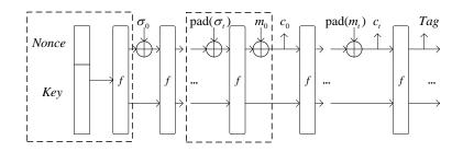
Fig. 3: Construction of GIMLI-CIPHER
