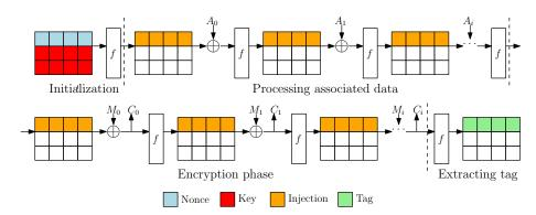
Fig. 17: Illustration of the AE scheme, where f is the Gimli permutation,  $A_i$  is the associated data block and  $M_i$  is the message block.
