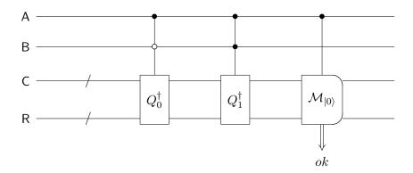
Figure 2: The quantum circuit  $V_{com}^{sup}$  that represents opening a quantum bit commitment by the honest receiver without measuring the opening information. The qubit A indicates whether this quantum bit commitment is to open, and the qubit B indicates the bit value to reveal. It outputs a single classical bit ok, which is equal to 1 if the quantum bit commitment is opened successfully or not opened.
