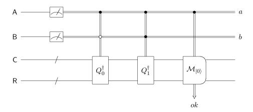
Figure 1: The quantum circuit  $V_{com}$  that represents opening a quantum bit commitment by the honest receiver. The classical bit a indicates whether this quantum bit commitment is to open, and the classical bit b indicates the bit value to reveal. It outputs a single classical bit ok, which is equal to 1 if the quantum bit commitment is opened successfully or not opened.
