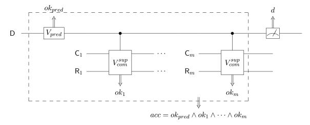
Figure 19: The quantum circuit obtained from the one depicted in Figure 7 by introducing more measurements
