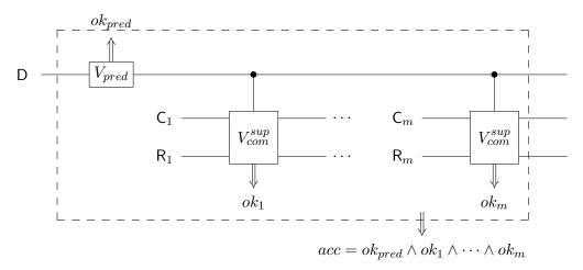
Figure 3: A typical verification involving opening quantum bit commitments, where arrows " $\uparrow$ " or " $\downarrow$ " indicate *classical* outputs. The classical bit  $ok_{pred}$  indicates whether the predicate check passes; each classical bit  $ok_i (1 \le i \le m)$  is equal to 1 if the *i*-th quantum bit commitment is opened successfully or not opened.
