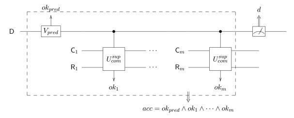
Figure 7: A typical verification involving opening quantum bit commitments (in the dashed box), with a posterior measurement of the opening register
