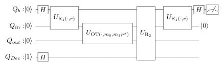
One can undone the register  $Q_{out}$  by a second application of OT function as depicted in the circuit below. But since  $m_0, m_1$  and the randomness r' are not known to the receiver, this second application also has to be applied by the sender. Therefore, we will end up making two quantum queries to the sender that is trivially useless. We depict the circuit below that uses two queries to the
