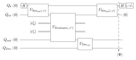
If the measurement returns 0, then the adversary outputs that the inputs of the sender are the same. Otherwise, it outputs that the inputs are different. The output of the circuit right before the application of the Hadamard operator is:
