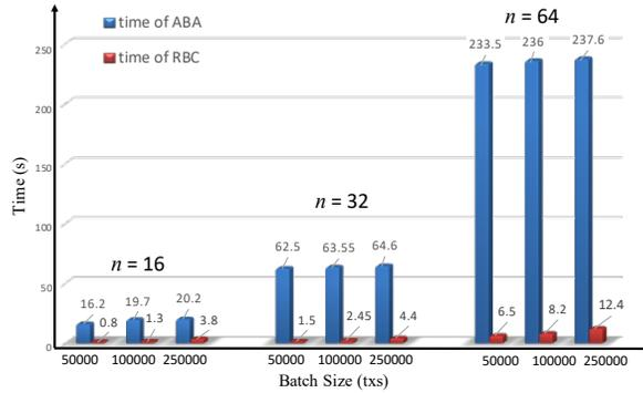
Fig. 2. Time costs of RBC and ABA in HoneyBadgerBFT, we get the running time of RBC by starting a timer when protocol starts and ending the timer when nodes get the output of RBC, averaging among multiple nodes and instances. The time of ABA is taking the maximum among all ABA instances a node needs to run.
