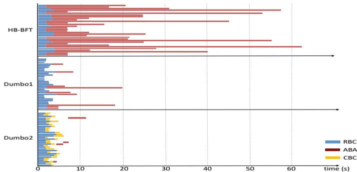
Fig. 5. Running time breakdown of Dumbo1/2 and HoneyBadgerBFT on one random node <sup>5</sup>.
