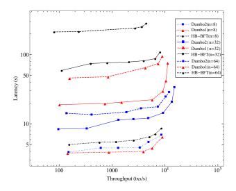
Fig. 8. Throughput vs. Latency
